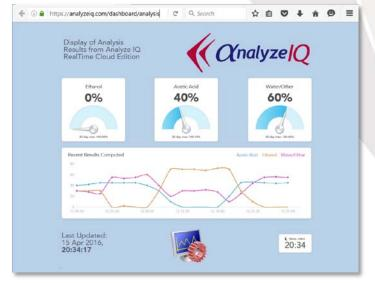
Analyze IQ RealTime is configured to run as a separate process from the client's software, and the two software programs interact using standard inter-process communications and XML-formatted messages. This design allows Analyze IQ RealTime to interact with client software developed using virtually any PC-supported software development framework and language. It can also be configured to run as a service on a desktop PC, or on a cloud server.
